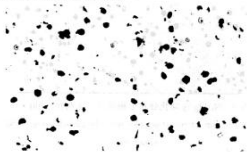
图4 不加 Sn, 用镍镁球化剂处理的球铁组织 100\times Fig.4 Microstructure of ductile iron treated by Ni-Mg nodularizer
