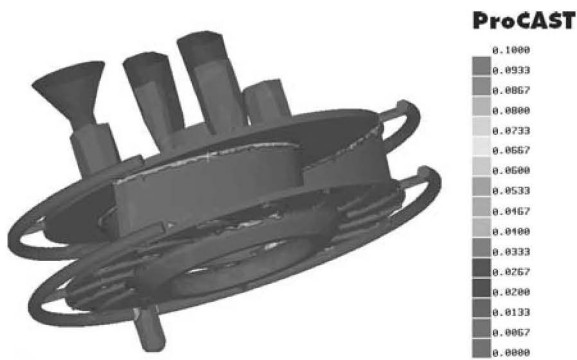
图8 上盖板和叶片交接处可能出现热裂 Fig. 8 Hot tearing may occur at the junction of upper cover plate and blade
