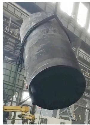
图8 百吨级球墨铸铁核乏燃料容器铸件 Fig. 8 100-ton grade ductile iron casting container of the spent nuclear fuel
