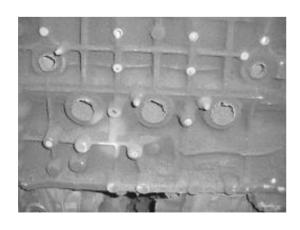
图3 缸体左侧面气孔 Fig. 3 Gas blowhole on the left side of cylinder
