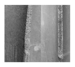
图4 两种砂芯涂料浸渗深度对比 Fig. 4 Penetration depth comparison between the two sand core coatings
