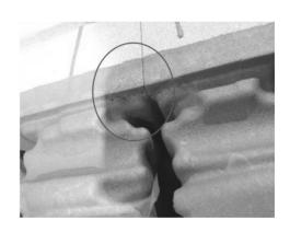
图6 缸体曲轴箱芯涂料层 Fig. 6 Coating layer of cylinder crankcase core
