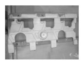
图8 浸涂后的油道砂芯 Fig. 8 Oil channel sand core after dip coating
