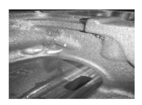
图5 缸体局部粘砂 Fig. 5 Burning-on defect on the surface of cylinder casting
