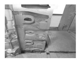
图7 油道粘砂铸件 Fig. 7 Casting with burn-on in oil channel
