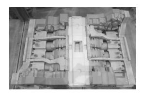
图2 国**VI**缸体砂芯(水套砂芯采用86<sup>#</sup>涂料) Fig. 2 National VI cylinder core ( water jacket core using 86<sup>#</sup> coating )
