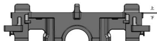
图4 轴承箱分型方案 Fig. 4 Parting scheme of bearing box casting
