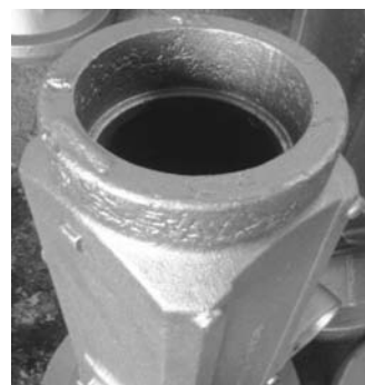
图4 皱皮缺陷 Fig. 4 Elephant skin defect
