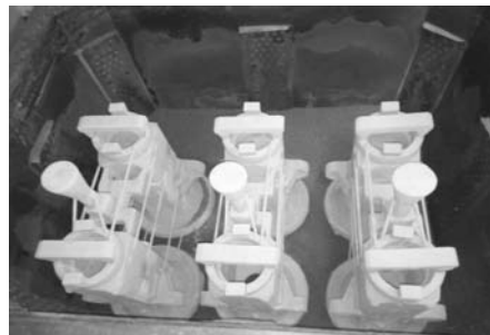
图7 串铸工艺装箱 Fig. 7 Layout of yellow patterns in molding box using cluster casting process
