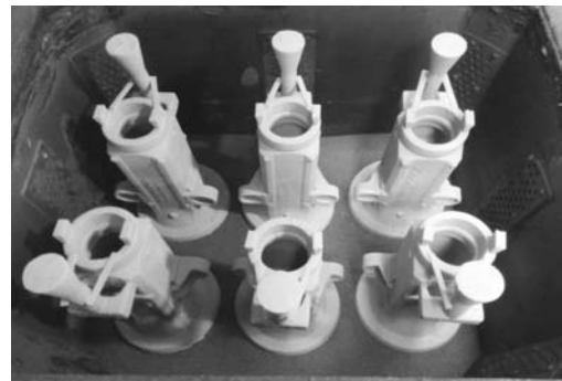
图3 黄模装箱 Fig. 3 Layout of yellow patterns in molding box
