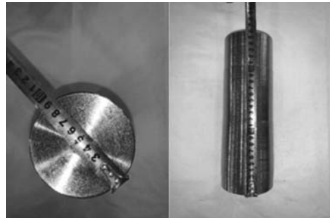
图1 15 kg级Ni-Ti-Zr形状记忆合金铸锭照片 Fig. 1 Photos of Ni-Ti-Zr shape memory alloy ingot weighing up to 15 kg
