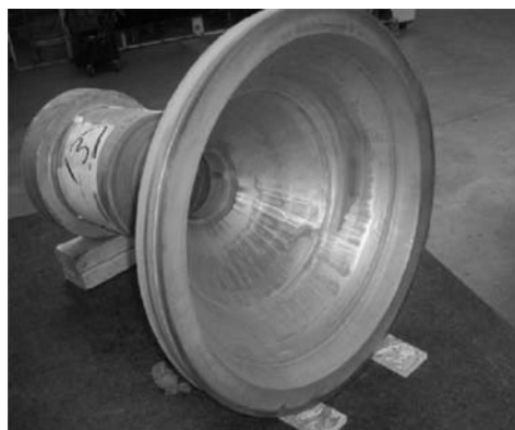
图3 Synertech PM公司开发的Ti-6Al-4V发动机大型框架部件 Fig. 3 Large engine frame parts made of Ti-6Al-4V developed by Synertech PM company
