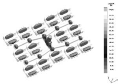
图3 铸件凝固60%时的液相区显示 Fig. 3 Display of liquid phase region with casting solidification up to 60%
