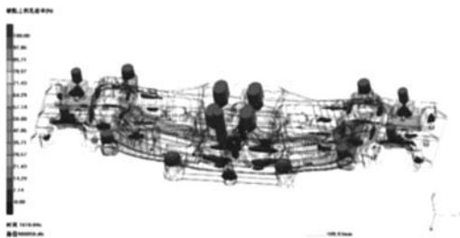
图9 改进冷铁工艺后凝固模拟结果 Fig. 9 Simulation results of casting solidification process after chill placing improved
