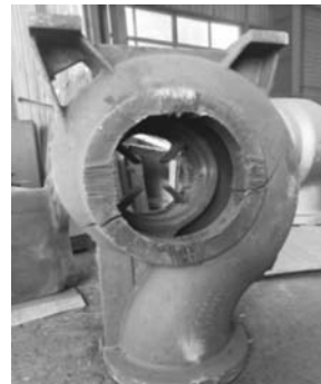
图2 泵体类铸件裂纹缺陷图 Fig. 2 Pump casting with cracks
