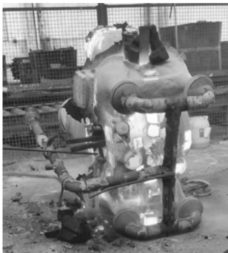
图6 铸件打箱后强制风冷 Fig. 6 Forced air cooling for casting after shaking out from mold
