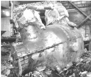
图7 打箱后铸件 Fig. 7 Valve casting with gating system
