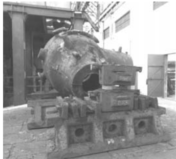
图8 铸件装炉热处理 Fig. 8 Valve casting without gating system
