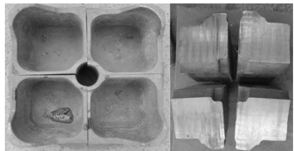
图5 心盘铸件及其解剖图 Fig. 5 Produced center plate casting and its dissection picture
